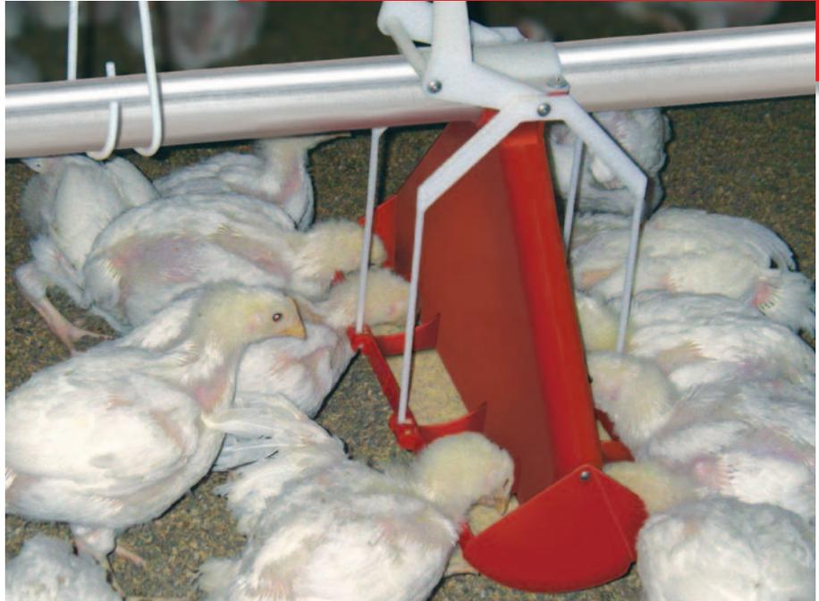
The first true perimeter feeder, the Butterfly® feeder gives birds full access to feed while keeping them out of the trays.
