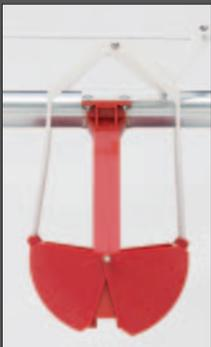
With a half turn of the winch, all feeders on a line open up simultaneously for feed removal and cleaning.
